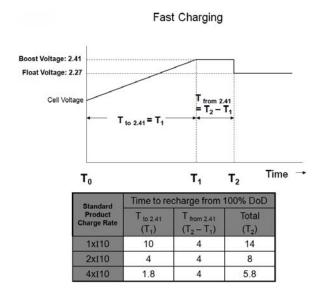
The table above shows the time needed to recharge following a 100% DOD cycle,
