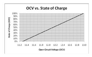
The graph shows that a healthy, fully charged NSB automotive and marine battery will have an OCV of approximately 13.0 V.
